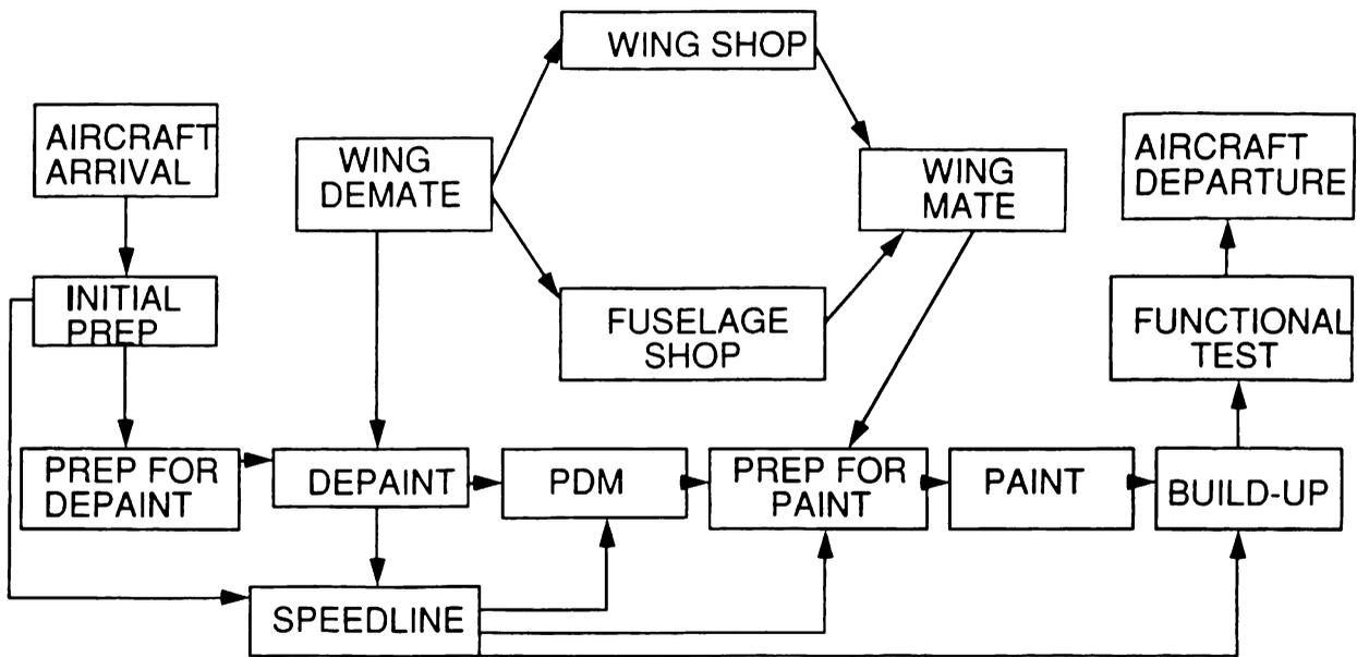
Figure 2: Programmed Depot Maintenance (PDM) Process with Speedline and Center Wing Box Replacement Included
