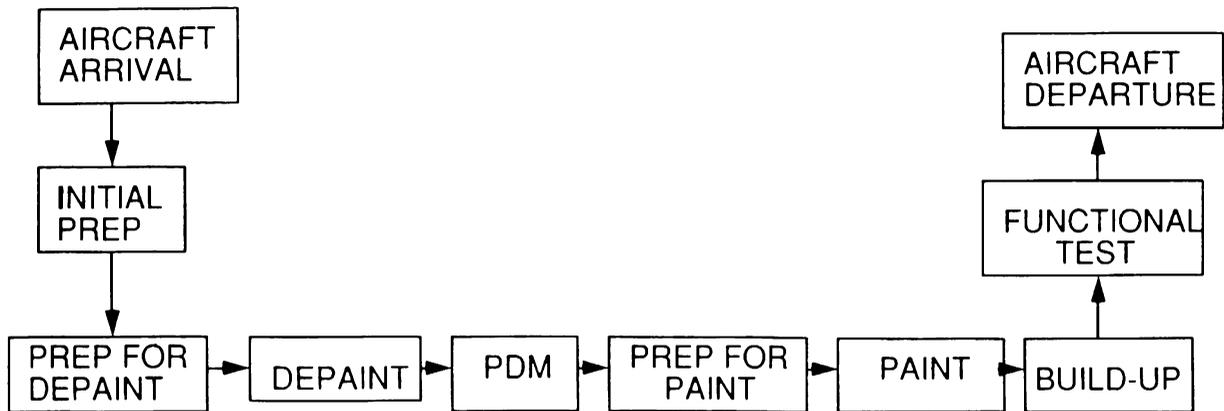
Figure 1: Initial Programmed Depot Maintenance (PDM) Process
