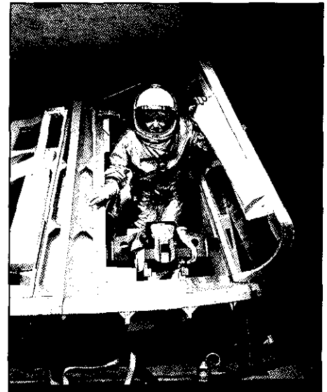
Under weightless conditions, a tester evaluates ways of exiting a model of a space capsule.
