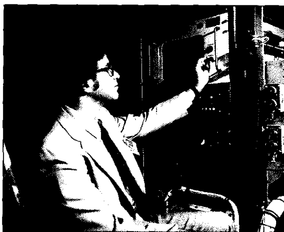
The C-130 test bed carried the AN/APD-10 Synthetic Aperture Radar Bistatic receiver for the TBIRD program.
